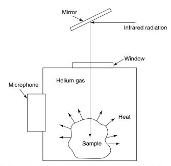
**Figure 2.18** Schematic of a typical photoacoustic spectroscopy cell. From Stuart, B., *Modern Infrared Spectroscopy*, ACOL Series, Wiley, Chichester, UK, 1996. © University of Greenwich, and reproduced by permission of the University of Greenwich.
