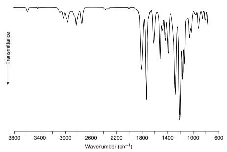
**Figure 4.13** Infrared spectrum of vanillin (cf. SAQ 4.8). From Stuart, B., *Biological Applications of Infrared Spectroscopy*, ACOL Series, Wiley, Chichester, UK, 1997. © University of Greenwich, and reproduced by permission of the University of Greenwich.
