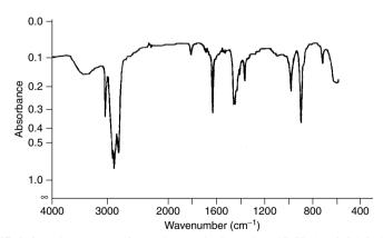
**Figure 4.17** Infrared spectrum of an unknown hydrocarbon ( $C_8H_{16}$ ) (cf. SAQ 4.12). From Stuart, B., *Modern Infrared Spectroscopy*, ACOL Series, Wiley, Chichester, UK, 1996. © University of Greenwich, and reproduced by permission of the University of Greenwich.
