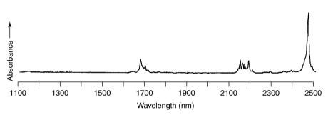
**Figure 4.10** NIR spectrum of benzene (cf. SAQ 4.7). From Weyer, L. G. and Lo, S. C., 'Spectra–Structure Correlations in the Near-Infrared', in *Handbook of Vibrational Spectroscopy*, Vol. 3, Chalmers, J. M. and Griffiths, P. R. (Eds), pp. 1817–1837. Copyright 2002. © John Wiley & Sons Limited. Reproduced with permission.
