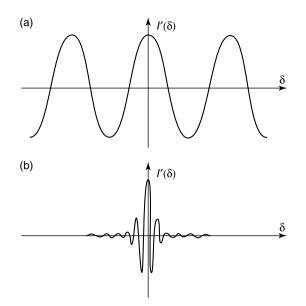
**Figure 2.5** Interferograms obtained for (a) monochromatic radiation and (b) polychromatic radiation. Reproduced with permission from Barnes, A. J. and Orville-Thomas, W. J. (Eds), *Vibrational Spectroscopy – Modern Trends*, Elsevier, Amsterdam, Figure 2, p. 55 (1977).
