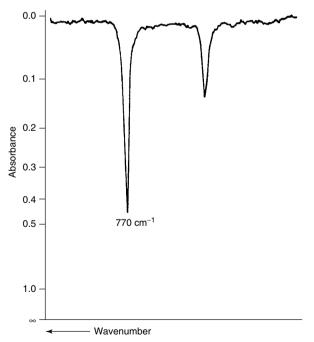
**Figure 3.12** Infrared spectrum of *m*-xylene in cyclohexane (2 vol%, 0.1 mm pathlength). From Stuart, B., *Modern Infrared Spectroscopy*, ACOL Series, Wiley, Chichester, UK, 1996. © University of Greenwich, and reproduced by permission of the University of Greenwich.
