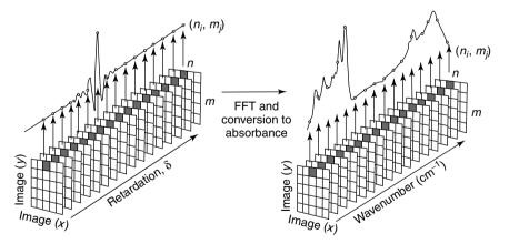
**Figure 2.21** FTIR imaging data set. From Kidder, L. H., Levin, I. W. and Lewis, E. N., 'Infrared Spectroscopic Imaging Microscopy: Applications to Biological Systems', in *Proceedings of the 11th International Fourier Transform Spectroscopy Conference*, Athens, GA, USA, August 10–15, 1997, de Haseth, J. A. (Ed.), Figure 1, p. 148, American Institute of Physics, Melville, New York, 1998, pp. 148–158. Reproduced by permission of American Institute of Physics.
