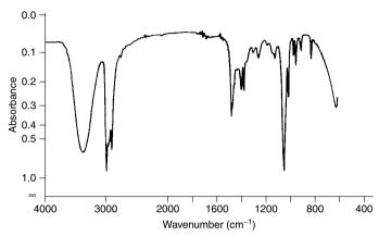
**Figure 4.16** Infrared spectrum of an unknown liquid ( $C_4H_{10}O$ ) (cf. SAQ 4.11). From Stuart, B., *Modern Infrared Spectroscopy*, ACOL Series, Wiley, Chichester, UK, 1996. © University of Greenwich, and reproduced by permission of the University of Greenwich.
