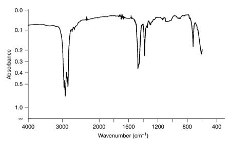
**Figure 4.15** Infrared spectrum of an unknown hydrocarbon ( $C_{10}H_{22}$ ) (cf. SAQ 4.10). From Stuart, B., *Modern Infrared Spectroscopy*, ACOL Series, Wiley, Chichester, UK, 1996. © University of Greenwich, and reproduced by permission of the University of Greenwich.
