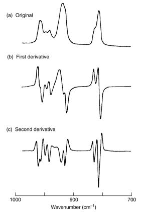
**Figure 3.7** Complex absorption band (a), plus corresponding first (b) and second (c) derivatives. From *Perkin-Elmer Application Notes on Derivative Spectroscopy*, Perkin-Elmer, Norwalk, CT, USA, 1984, and reproduced with permission of the Perkin-Elmer Corporation.
