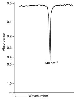
**Figure 3.11** Infrared spectrum of *o*-xylene in cyclohexane (1 vol%, 0.1 mm pathlength). From Stuart, B., *Modern Infrared Spectroscopy*, ACOL Series, Wiley, Chichester, UK, 1996. © University of Greenwich, and reproduced by permission of the University of Greenwich.
