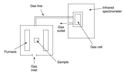
Figure 2.23 Layout of a typical thermal analysis-infrared spectroscopy system.
