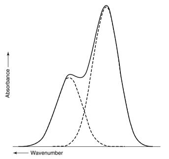
Figure 3.9 Illustration of curve-fitting of overlapping infrared bands.
