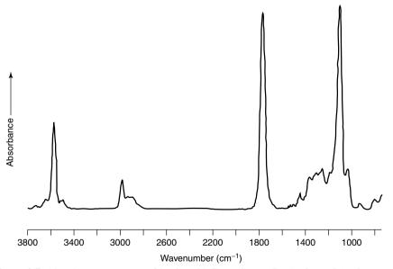
**Figure 2.7** Absorbance spectrum of lactic acid. From Stuart, B., *Biological Applications of Infrared Spectroscopy*, ACOL Series, Wiley, Chichester, UK, 1997. © University of Greenwich, and reproduced by permission of the University of Greenwich.
