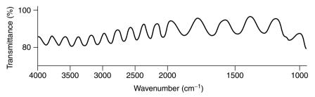
**Figure 2.13** Interference pattern recorded with an empty cell in the sample beam. From Stuart, B., *Modern Infrared Spectroscopy*, ACOL Series, Wiley, Chichester, UK, 1996. © University of Greenwich, and reproduced by permission of the University of Greenwich.
