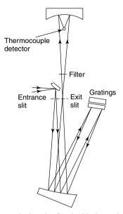
**Figure 2.1** Schematic of the optical path of a double-beam infrared spectrometer with a grating monochromator. Reproduced from Brittain, E. F. H., George, W. O. and Wells, C. H. J., *Introduction to Molecular Spectroscopy*, Academic Press, London, Copyright (1975), with permission from Elsevier.
