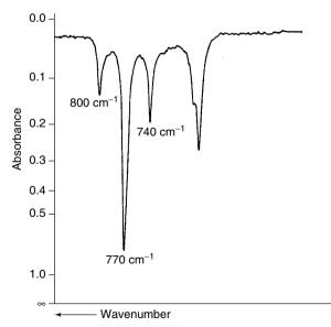
**Figure 3.14** Infrared spectrum of commercial xylene in cyclohexane (5 vol%, 0.1 mm pathlength). From Stuart, B., *Modern Infrared Spectroscopy*, ACOL Series, Wiley, Chichester, UK, 1996. © University of Greenwich, and reproduced by permission of the University of Greenwich.
