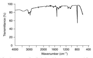
**Figure 4.4** Infrared spectrum of a disubstituted benzene: compound B (cf. SAQ 4.3). From Stuart, B., *Modern Infrared Spectroscopy*, ACOL Series, Wiley, Chichester, UK, 1996. © University of Greenwich, and reproduced by permission of the University of Greenwich.
