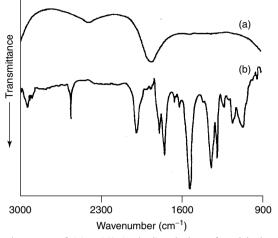
**Figure 3.5** Infrared spectra of (a) a 1% (wt/vol) solution of aspirin in water and (b) the same solution after subtraction of the water spectrum. From Stuart, B., *Modern Infrared Spectroscopy*, ACOL Series, Wiley, Chichester, UK, 1996. © University of Greenwich, and reproduced by permission of the University of Greenwich.
