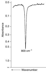
**Figure 3.13** Infrared spectrum of *p*-xylene in cyclohexane (2 vol%, 0.1 mm pathlength). From Stuart, B., *Modern Infrared Spectroscopy*, ACOL Series, Wiley, Chichester, UK, 1996. © University of Greenwich, and reproduced by permission of the University of Greenwich.
