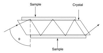
**Figure 2.15** Schematic of a typical attenuated total reflectance cell. From Stuart, B., *Modern Infrared Spectroscopy*, ACOL Series, Wiley, Chichester, UK, 1996. © University of Greenwich, and reproduced by permission of the University of Greenwich.
