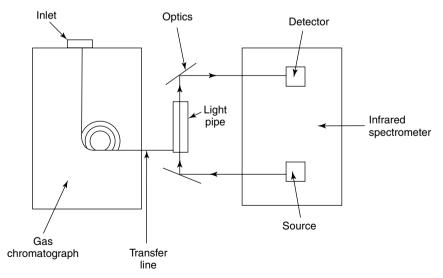
Figure 2.22 Layout of a typical GC-IR system.
