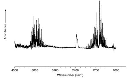
**Figure 2.2** Infrared spectrum of atmospheric contributions (e.g.  $CO_2$  and  $H_2O$ ). From Stuart, B., *Modern Infrared Spectroscopy*, ACOL Series, Wiley, Chichester, UK, 1996. © University of Greenwich, and reproduced by permission of the University of Greenwich.
