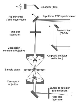
Figure 2.19 Layout of a typical FTIR microspectrometer. Reprinted from Katon, J. E., Sommer, A. J. and Lang, P. L., *Applied Spectroscopy Reviews*, Vol. 25, pp. 173–211 (1989–1990), courtesy of Marcel Dekker, Inc.
