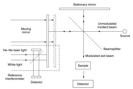
Figure 2.4 Schematic of a Michelson interferometer. From Stuart, B., *Modern Infrared Spectroscopy*, ACOL Series, Wiley, Chichester, UK, 1996. © University of Greenwich, and reproduced by permission of the University of Greenwich.
