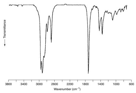
Figure 4.11 Infrared spectrum of citronellal. From Stuart, B., *Biological Applications* of *Infrared Spectroscopy*, ACOL Series, Wiley, Chichester, UK, 1997. © University of Greenwich, and reproduced by permission of the University of Greenwich.
