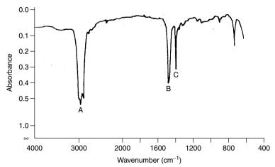
**Figure 4.1** Infrared spectrum of nonane  $(C_9H_{20})$  (cf. SAQ 4.1). From Stuart, B., *Modern Infrared Spectroscopy*, ACOL Series, Wiley, Chichester, UK, 1996. © University of Greenwich, and reproduced by permission of the University of Greenwich.
