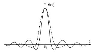
**Figure 2.6** Instrument lineshape without apodization. Reproduced with permission from Barnes, A. J. and Orville-Thomas, W. J. (Eds), *Vibrational Spectroscopy – Modern Trends*, Elsevier, Amsterdam, Figure 3, p. 55 (1977).
