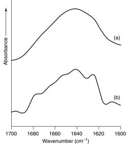
**Figure 3.8** Broad infrared band (a) before and (b) after deconvolution. From Stuart, B., *Modern Infrared Spectroscopy*, ACOL Series, Wiley, Chichester, UK, 1996. © University of Greenwich, and reproduced by permission of the University of Greenwich.
