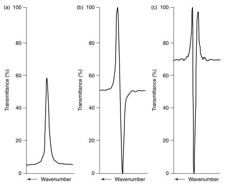
**Figure 3.6** Differentiation of spectra: (a) single absorption peak; (b) first derivative; (c) second derivative. From Stuart, B., *Modern Infrared Spectroscopy*, ACOL Series, Wiley, Chichester, UK, 1996. © University of Greenwich, and reproduced by permission of the University of Greenwich.
