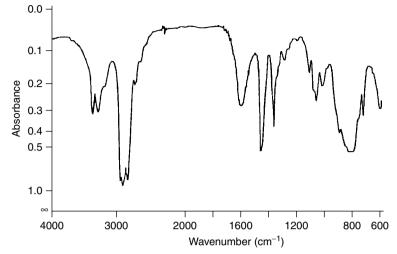
**Figure 4.8** Infrared spectrum of hexylamine (cf. SAQ 4.5). From Stuart, B., *Modern Infrared Spectroscopy*, ACOL Series, Wiley, Chichester, UK, 1996. © University of Greenwich, and reproduced by permission of the University of Greenwich.
