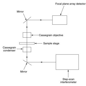
Figure 2.20 Layout of a typical FTIR imaging microspectrometer.
