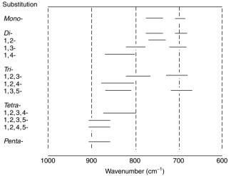
**Figure 4.2** Out-of-plane bending vibrations of aromatic compounds. From Stuart, B., *Modern Infrared Spectroscopy*, ACOL Series, Wiley, Chichester, UK, 1996. © University of Greenwich, and reproduced by permission of the University of Greenwich.
