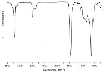
**Figure 2.8** Transmittance spectrum of lactic acid. From Stuart, B., *Biological Applications of Infrared Spectroscopy*, ACOL Series, Wiley, Chichester, UK, 1997. © University of Greenwich, and reproduced by permission of the University of Greenwich.
