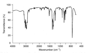
**Figure 4.3** Infrared spectrum of a disubstituted benzene: compound A (cf. SAQ 4.3). From Stuart, B., *Modern Infrared Spectroscopy*, ACOL Series, Wiley, Chichester, UK, 1996. © University of Greenwich, and reproduced by permission of the University of Greenwich.
