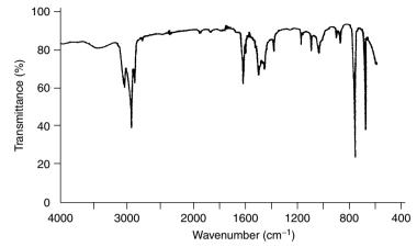
**Figure 4.5** Infrared spectrum of a disubstituted benzene: compound C (cf. SAQ 4.3). From Stuart, B., *Modern Infrared Spectroscopy*, ACOL Series, Wiley, Chichester, UK, 1996. © University of Greenwich, and reproduced by permission of the University of Greenwich.
