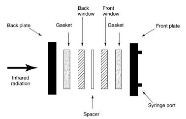
**Figure 2.9** Schematic of a typical semi-permanent liquid cell. From Stuart, B., *Biological Applications of Infrared Spectroscopy*, ACOL Series, Wiley, Chichester, UK, 1997. © University of Greenwich, and reproduced by permission of the University of Greenwich.
