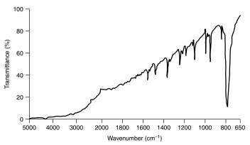
Figure 2.11 Infrared spectrum of a mull (cf. SAQ 2.3). From Stuart, B., *Modern Infrared Spectroscopy*, ACOL Series, Wiley, Chichester, UK, 1996. © University of Greenwich, and reproduced by permission of the University of Greenwich.
