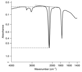
**Figure 3.4** An example of a baseline correction. From Stuart, B., *Modern Infrared Spectroscopy*, ACOL Series, Wiley, Chichester, UK, 1996. © University of Greenwich, and reproduced by permission of the University of Greenwich.
